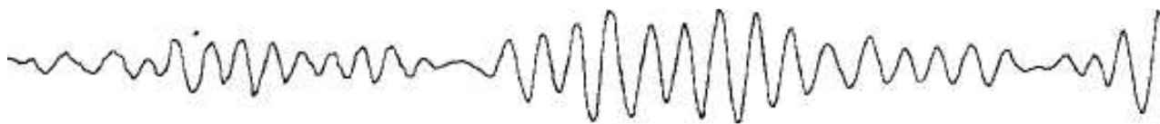
Fig. 15. Horizontal oscillations of the 9th floor of a residential building: street Matrosov
