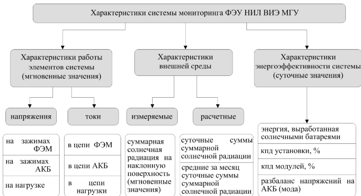
Рис. 1. Состав характеристик, определяемых системой мониторинга ФЭУ НИЛ ВИЭ МГУ Fig. 1. The composition of the characteristics defined photovoltaic energy plant's monitoring system of the Renewable Energy Scientific Research Laboratory of the Moscow State University (RESRL of the MSU)
